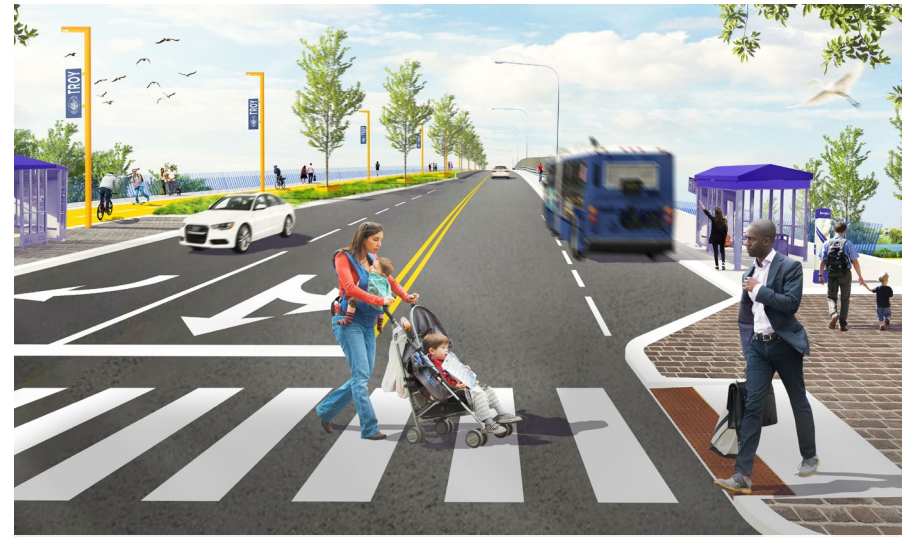
This rendering illustrates the new eastbound approach of the intersection, including the curb extensions, bus stops, and shared use path along the southside of the bridge.
