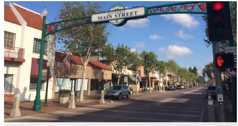
Example slow street - common elements include reduction or elimination of curbs and textured or colored surfaces
